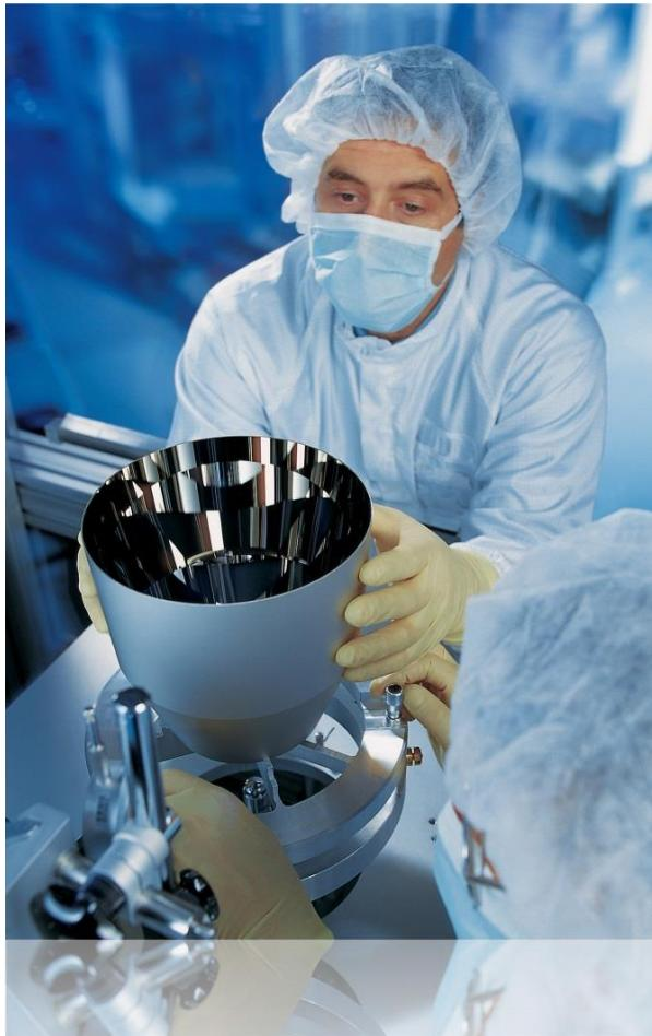
EUV mirrors are polished to an accuracy of ~50 picometers – less than the diameter of a silicon atom.
